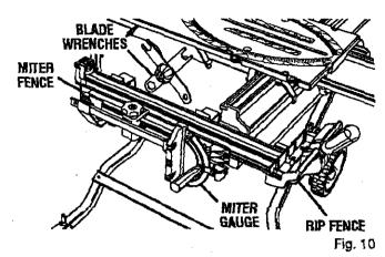
Stand facing the back of the table saw. The longest part of the miter table base must be stored to the left. To secure the sliding miter table:
